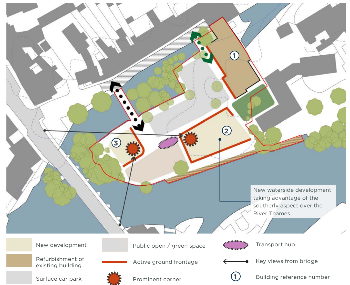
Fig 10.27: Plan setting out the key design principles for redevelopment of the Upper Reaches Site.
